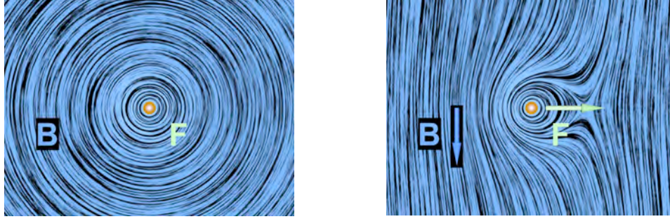
Figure 8.6.1 Two frames of an animation of the magnetic field around a positive charge moving out of the page in a time-changing magnetic field that points downward. The blue vector is the magnetic field and the green vector is the force on the point charge.
