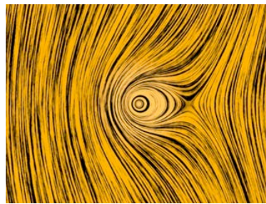
Figure 1.4.7 A constant downward flow interacting with a counter-clockwise circulating flow.
