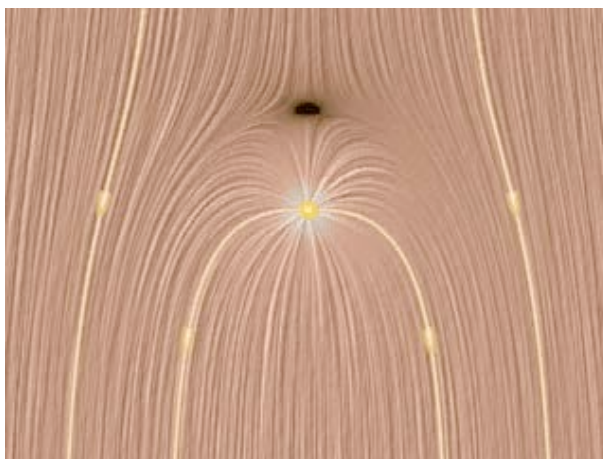
Figure 1.8.5: One frame of a movie showing the electric field lines of a positive charge moving upward in a downward constant field. The motion of the field lines and texture patterns in this movie are in the direction of \vec{E} \times \vec{B} .
